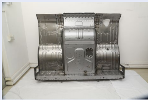
Assembly Sub Structure with Floor
